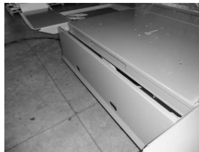
Diagram 7 / 8: Interim drive over ramp in the basic position / interim drive over ramp is folded down.
