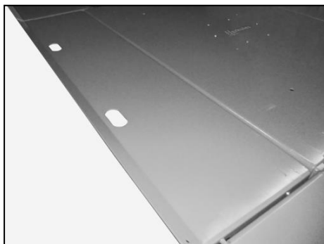
Picture 7 / 8: Interim drive over ramp in the basic position / interim drive over ramp is folded down.
