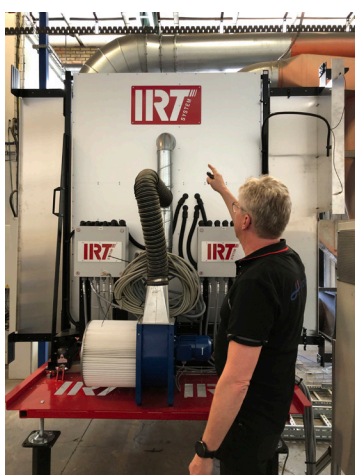
Small footprint. This model 2.3x2.8 m (7.4x9.2 ft). Legs adjust height to conveyor position.
